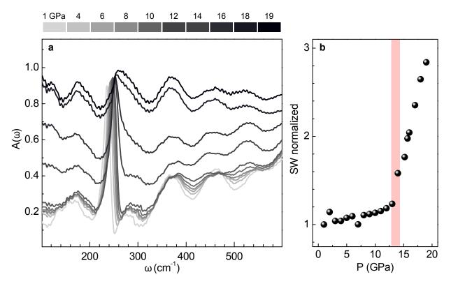
Figure 2. (a) Absorbance spectra at selected pressure values over the range  $[1 \div 19]$  GPa. (b) Normalized spectral weight  $SW(P, P_0)$  (see text); the red vertical stripe highlights the pressure range where the change of slope occurs.
