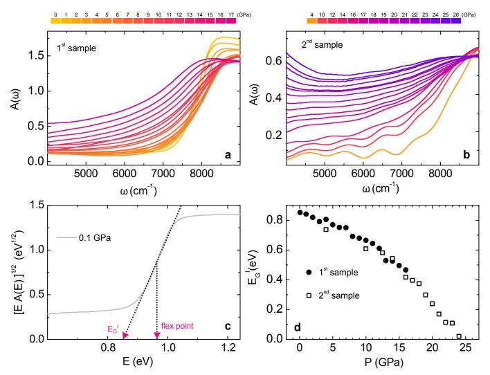
Figure 1. (a) Absorbance spectra collected in the first run over the  $[0,1 \div 17]$  GPa range. (b) Absorbance spectra collected in the second run over the  $[4 \div 27]$  GPa range. (c) Tauc-plot at P = 0.1 GPa and linear extrapolation of the energy gap. (d) Energy gap as a function of the pressure for the first (dots) and the second (open squares) run.
