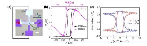
**Figure 4.** SOT of W/CGT bilayer at 150 K. a) Optical microscope image of the device and schematic of the SOT measurement.  $H_{\text{ext}}$  and *j* show the directions of applied external field and current. Scale bar: 5 µm. b)  $R_{\text{H}}$ -*H* curves with applied out-of-plane (oop) and in-plane (ip) magnetic field at 150 K. c) Normalized  $\Delta R_{\text{H}}$  as the function of current density applied to the device under 1 kOe and –1 kOe external field.
