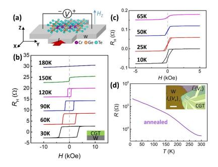
**Figure 1.** Transport measurements of  $T_{\rm C}$ -enhanced CGT. a) Schematic view of the device for the measurement of  $R_{\rm H}$ -H curves. b,c)  $R_{\rm H}$ -H curves of b) W/CGT and c) pristine CGT at selected temperatures. The inset of b) shows the bilayer structure. d) R-T curve of  $T_{\rm C}$ -enhanced CGT. The inset shows the microscope image and measurement setup.
