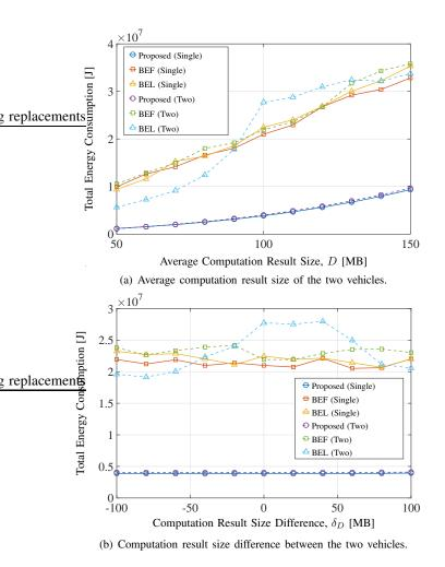
Fig. 5: Total energy consumption versus the average computation result size D and the computation result size difference  $\delta_D$  of two vehicles in the single-tier and two-tier network.
