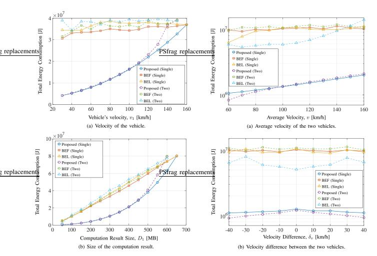
Fig. 3: Total energy consumption versus the velocity of the vehicle  $v_1$  and the computation result size of the vehicle  $D_1$  in the single-tier and two-tier network.
