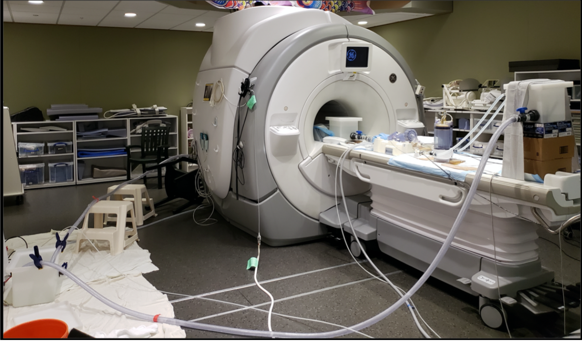
Figure 1: Experimental flow loop setup on the MRI magnet table in the Richard M. Lucas Center for Imaging at Stanford University.
