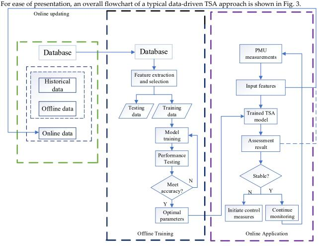
Fig. 3. Flowchart of a typical data-driven transient stability assessment method.
