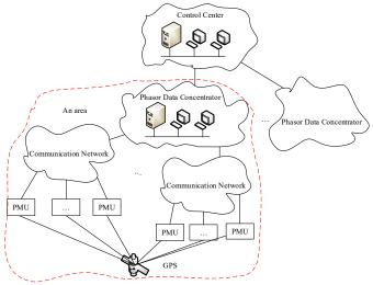
Fig. 2. Structure of WAMS
