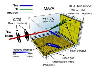
Figure 1: Schematic drawing of the detection set-up. A typical protontransfer reaction producing  $^{7}$ H with a  $^{19}$ F nucleus is also shown.
