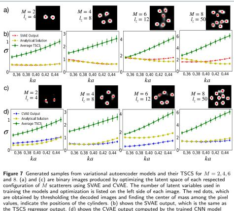
the TSCS regressor output. (d) shows the CVAE output computed by the trained CNN model from forward desired. The average TSCS for each wavenumber ka of 30 randomly selected training examples and their standard error is also plotted for comparison. While the semi-analytical solution does not match the regressor output completely, the optimized configurations clearly have much lower TSCS compared to the average TSCS.
