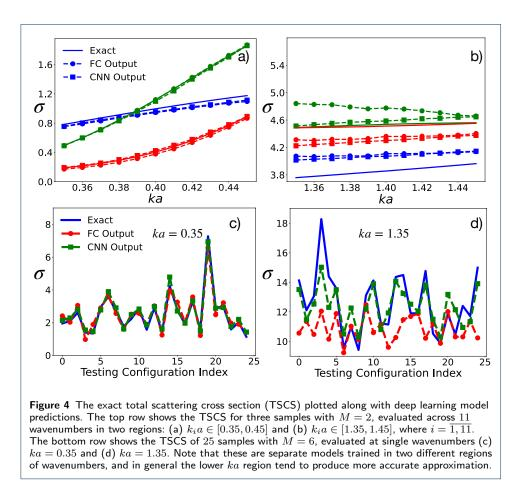
those obtained through the FC or the CNN. Note that the models are trained separately in the two regions of the wavenumber:  $k_i a \in [0.35, 045]$  and  $k_i a \in [1.35, 1.45]$ .
