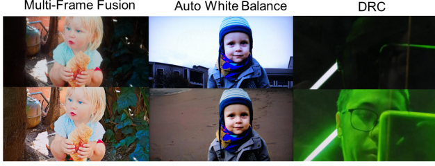
Figure S1. ISP non-linearity. The first column is brightness change caused by smartphone ISP multi-frame fusion. The dark part of background become bright after multi-frame fusion. The second column is smartphone ISP auto white balance operation. The boy face change from blue to yellow. The third column is smartphone ISP dynamic range correction, the image change from dark to bright.
