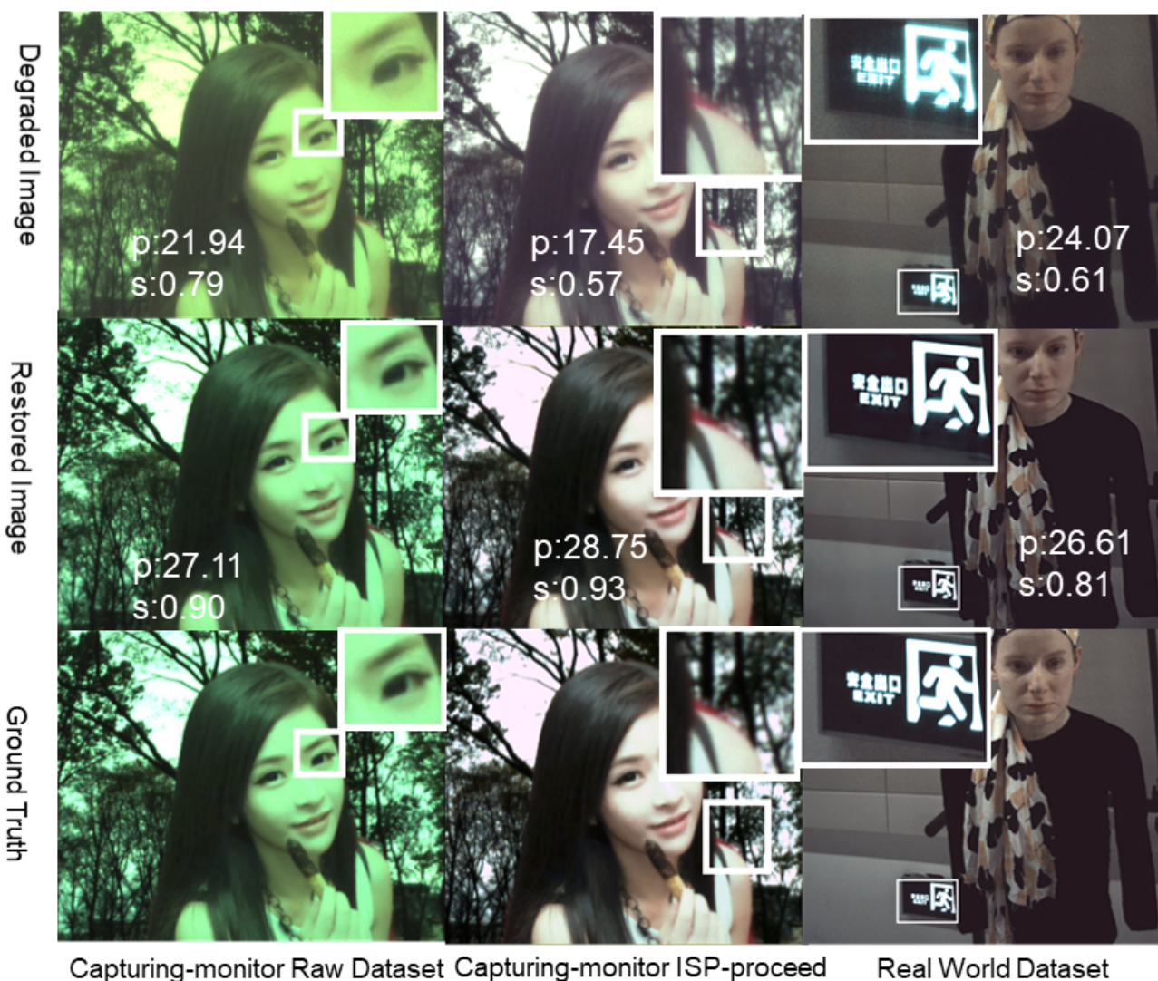
Figure S11. Restoration result. The first column is the monitor raw dataset restoration result. The restored raw image is processed by the legacy ISP, and the output is shown in the second column. The third column is real-world test result. We can see that there is obvious stripe-like diffraction artifacts in the green words in the third column degraded image, but removed in our result.
