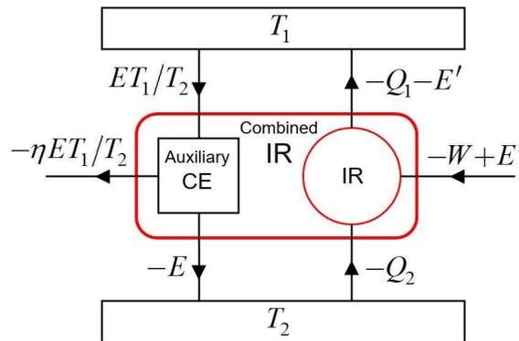
**Figure 4.** IR of Fig. 3(a) together with an auxiliary CE adjusted to reject the heat  $-E$  to the coldest reservoir. As no extra irreversibility is added by the CE, by imposing (9), the combined IR thus obtained is *indistinguishable* from that of Fig. 2(b).
