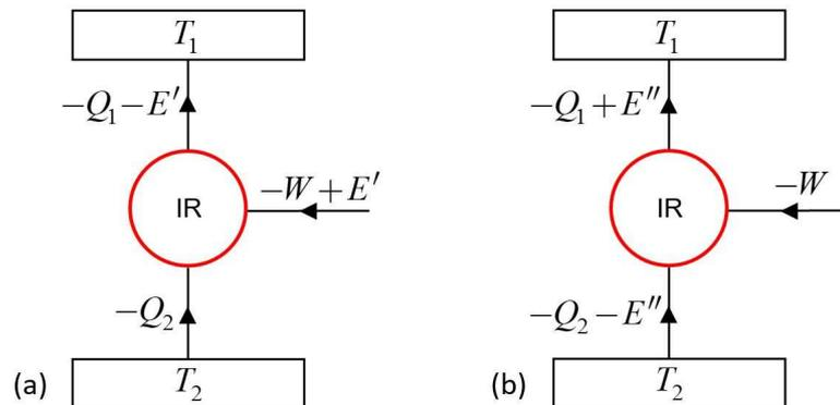
**Figure 3.** Alternatives for setting up the IR from the CR: (a) the heat  $-Q_2$  is kept the same; (b) the work  $-W$  is kept the same.  $E' > 0$  and  $E'' > 0$  relate to irreversibility.
