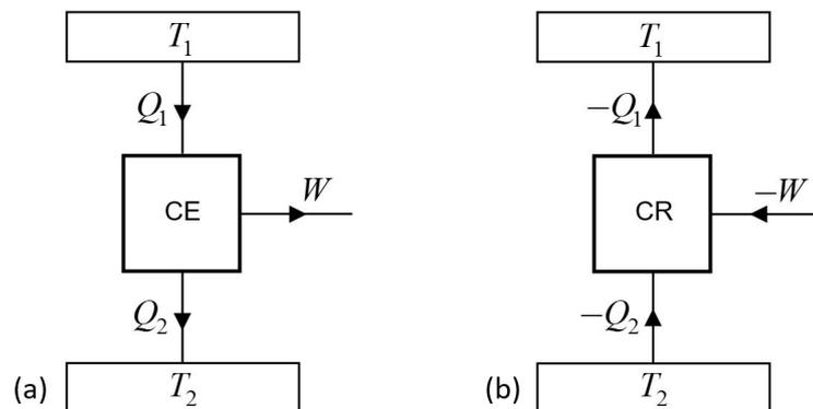
**Figure 1.** (a) Carnot engine (CE) and (b) Carnot refrigerator (CR), both operating between the reservoir temperatures  $T_1$  and  $T_2$ , with  $T_1 > T_2$ . As said in the text,  $Q_1 > 0$ ,  $Q_2 < 0$  and  $W < 0$ .
