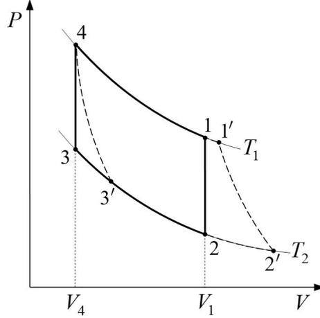
**Figure 6.** Pressure-volume diagram of the irreversible Stirling cycle 12341. The CE that absorbs the same heat  $Q_1$  at reservoir temperature  $T_1$  is the cycle 1'2'3'41'.
