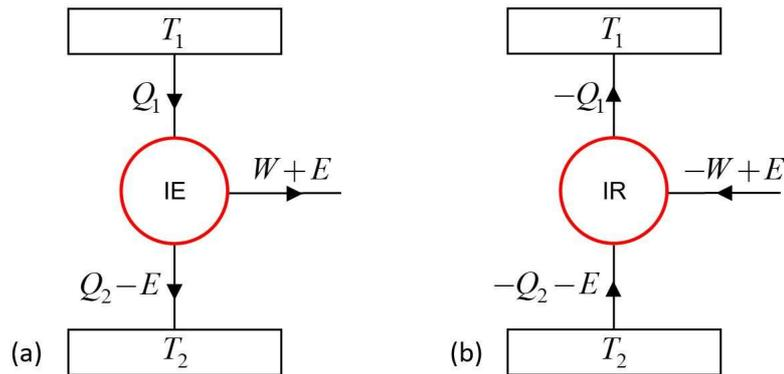
**Figure 2.** (a) IE and (b) IR, both operating between reservoir temperatures  $T_1$  and  $T_2$ , with  $T_1 > T_2$ . Absolute values of the heats exchanged with the hottest reservoir are equal and the same as that for the CE and CR.  $E > 0$  is related to the irreversibility.
