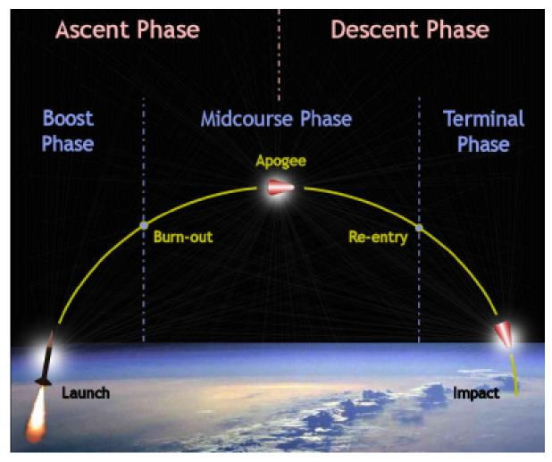
Figure 4. Flight path of Theater Ballistic Missiles [110]
