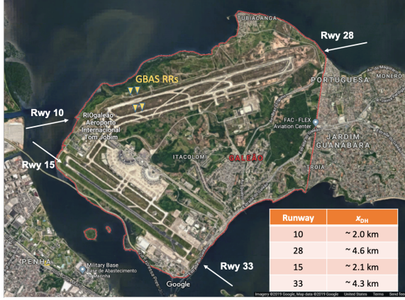
Fig. 2. x_{DH} values for Galeão airport. Each runway has a known x_{DH} location where an airplane reaches the minimum 200 ft decision height for a Category I precision approach.
