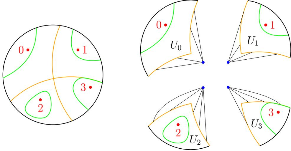
Figure 1: The minimum isolating cuts algorithm for  $|R| = 4$ . The orange marks the “upper boundary” of each green isolating cut. They are formed by the min-cut separating  $\{0, 1\}$  and  $\{2, 3\}$  and the min-cut separating  $\{0, 2\}$  and  $\{1, 3\}$ .
