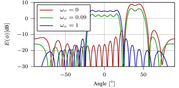
Fig. 3: Learned beampatterns (without hardware impairments) generated by the AE for different values of the hyper-parameter  $\omega_r$ , where the communication receiver and the radar target reside, respectively, in the intervals  $(30^\circ, 50^\circ)$  and  $(-20^\circ, 20^\circ)$ . The function  $E(\phi) = |\mathbf{a}_{\text{tx}}(\phi)^\top \mathbf{y}|^2$  accounts for how much energy is transmitted in a certain direction.
