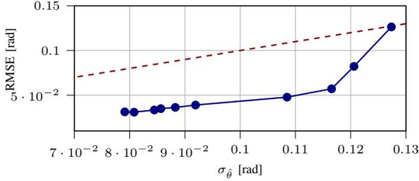
Fig. 4: Results (without hardware impairments) of the RMSE of the AoA against the associated standard deviation  $\sigma_{\hat{\theta}}$  for  $\omega_r \in \{0.01, 0.014, 0.015, 0.03, 0.09, 0.15, 0.4, 0.6, 0.7, 1\}$ . The dashed line shows  $\text{RMSE} = \sigma_{\hat{\theta}}$  as a reference.
