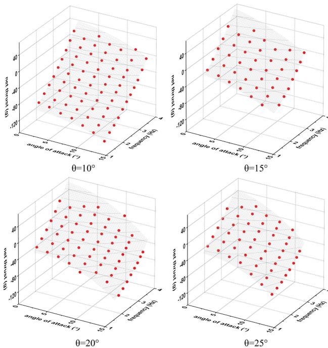
Fig. 10. Fitting surfaces of the cycle-averaged net thrust versus angle of attack and flapping frequency for different wrist mounting angles.
