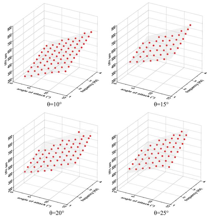
Fig. 10. Fitting surfaces of the cycle-averaged lift versus angle of attack and flapping frequency for different wrist mounting angles.
