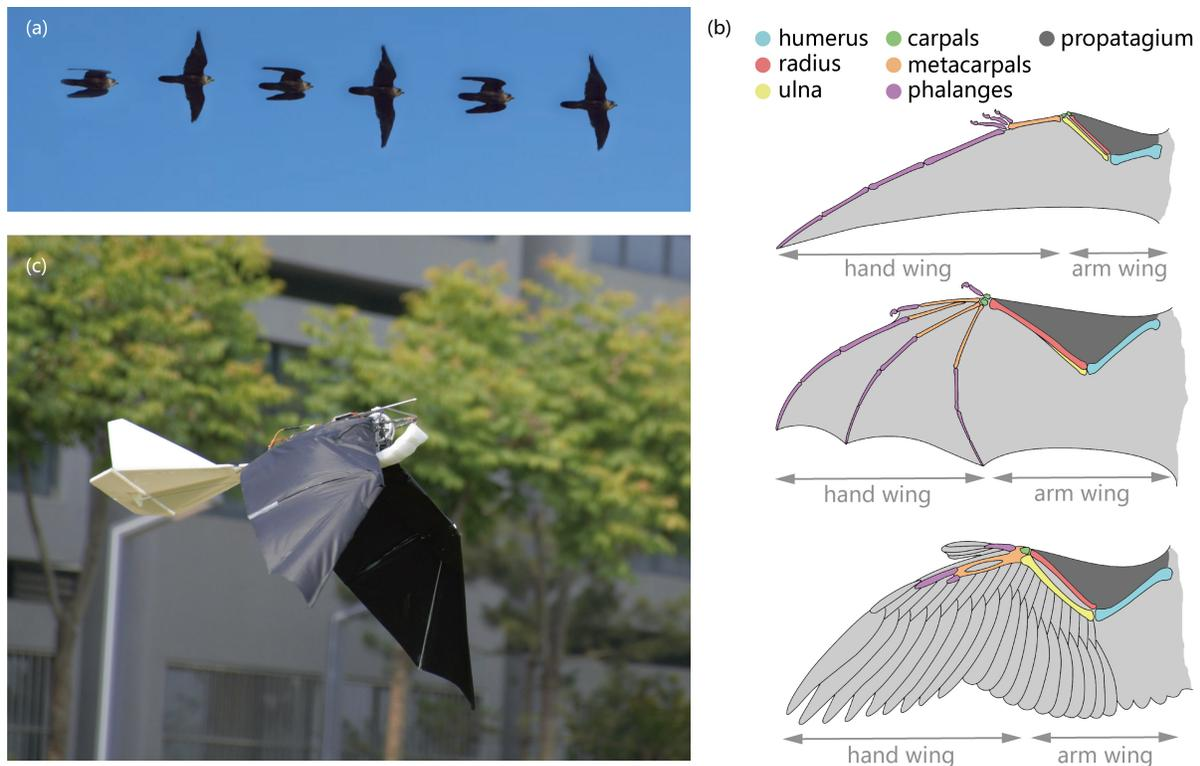
Fig. 1. The wingbeat pattern of avian and the forelimb anatomy of flying vertebrates inspired the design of a bionic FWAV. (a) Snapshot of a peregrine falcon during level flight. The wing is tucked in upstroke and extended in the downstroke. (b) Wing anatomy of pterosaur, bat, and bird, exhibiting analogous three-link structures. (c) The RoboFalcon FWAV in flight, as inspired by flying vertebrates, applying a novel actuation strategy for achieving the wingbeat pattern of the bird in (a).
