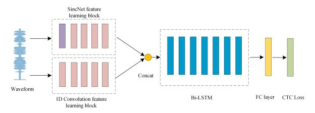
Fig. 1: The architecture of the proposed end-to-end automatic speech recognition system. The model consists of the feature learning block and the backbone network. A feature learning block is used to learn features from the raw waveforms.
