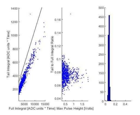
Figure 15: PSD plot of the static master 1U400 alpha source after a measurement time of 2 minutes.
