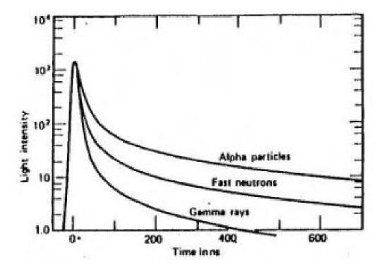
Figure 2: Effect of decay constants on the output light intensity in the liquid scintillator material. Credit: Knoll [11]
