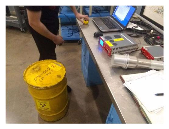
Figure 8: An image of the experimental PuBe PSD measurement setup.
