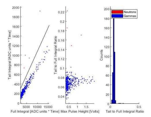
Figure 17: PSD plot of the background environment (the Pennsylvania State University's nuclear fuels building) in which the PuBe neutron source is measured. Measurement time is 5 seconds.
