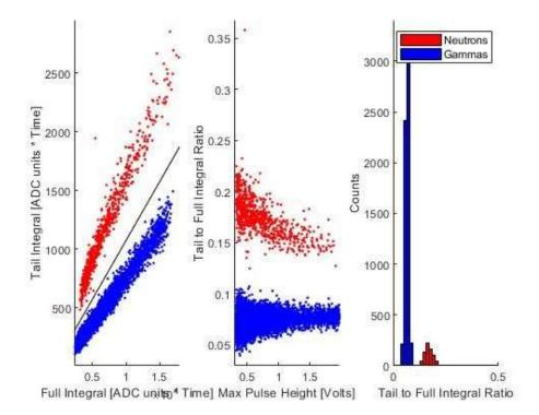
Figure 16: PSD plot of the PuBe neutron source after a measurement time of 5 seconds.
