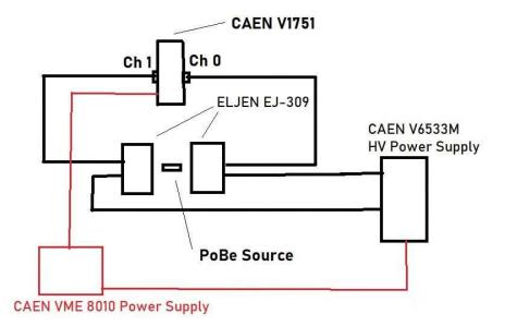
Figure 7: Schematic measurement setup for the PoBe coincidence measurement.
