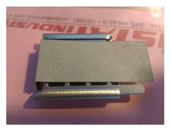
Figure 6: Image of the assembled Static Master 1U400 Self Powered ( $\alpha$ ,n) neutron source.
