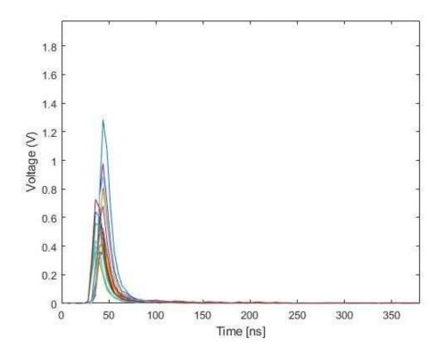
Figure 3: Plot of 20 PSD pulse waveforms from the PuBe neutron source utilized in this report.
