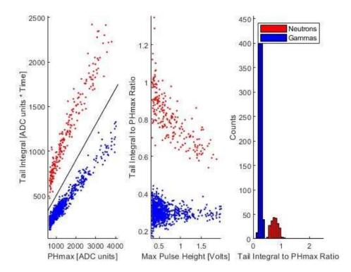
Figure 14: PSD plot of the PoBe neutron source after a measurement time of 2 minutes.
