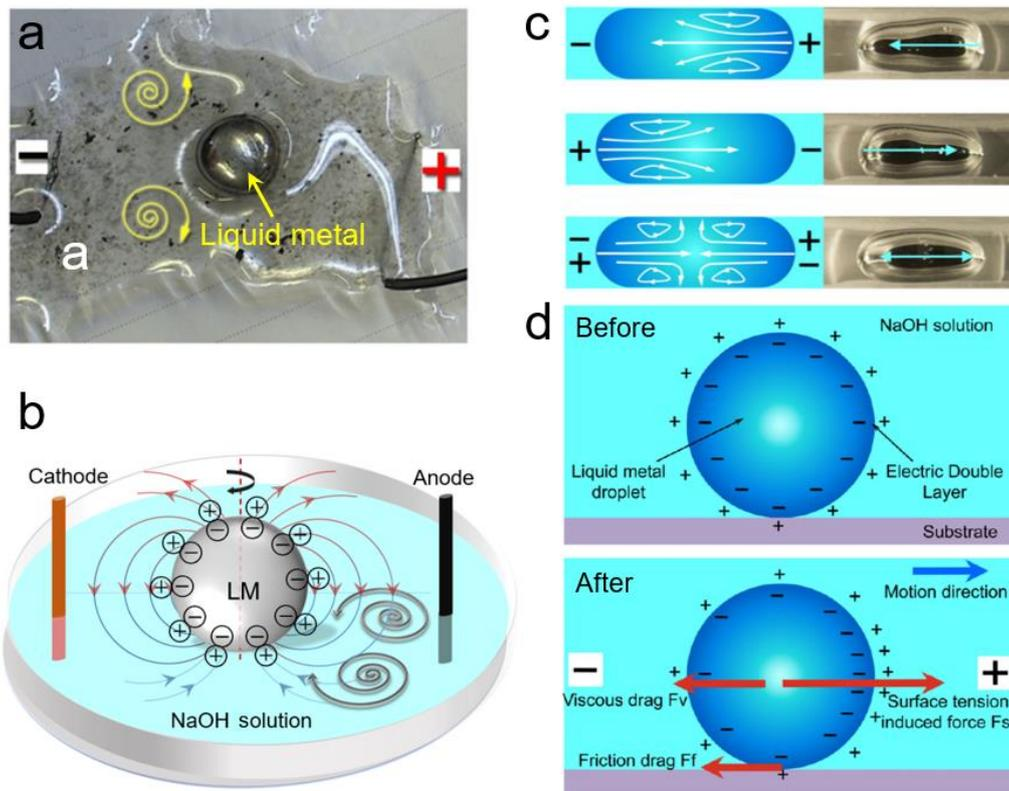
**Figure 5.** The rotation and transformation of liquid metal in the solution under an external electric field: (a) Experimental case of rotating liquid metal droplet under direct current<sup>[22]</sup>; (b) Schematic for rotating liquid metal droplet under direct current; (c) Resonant oscillation phenomenon of liquid metal droplet under matching alternating field; (d) Electric field on the liquid metal-electrolyte interface before and after applying external electric field<sup>[27]</sup>.
