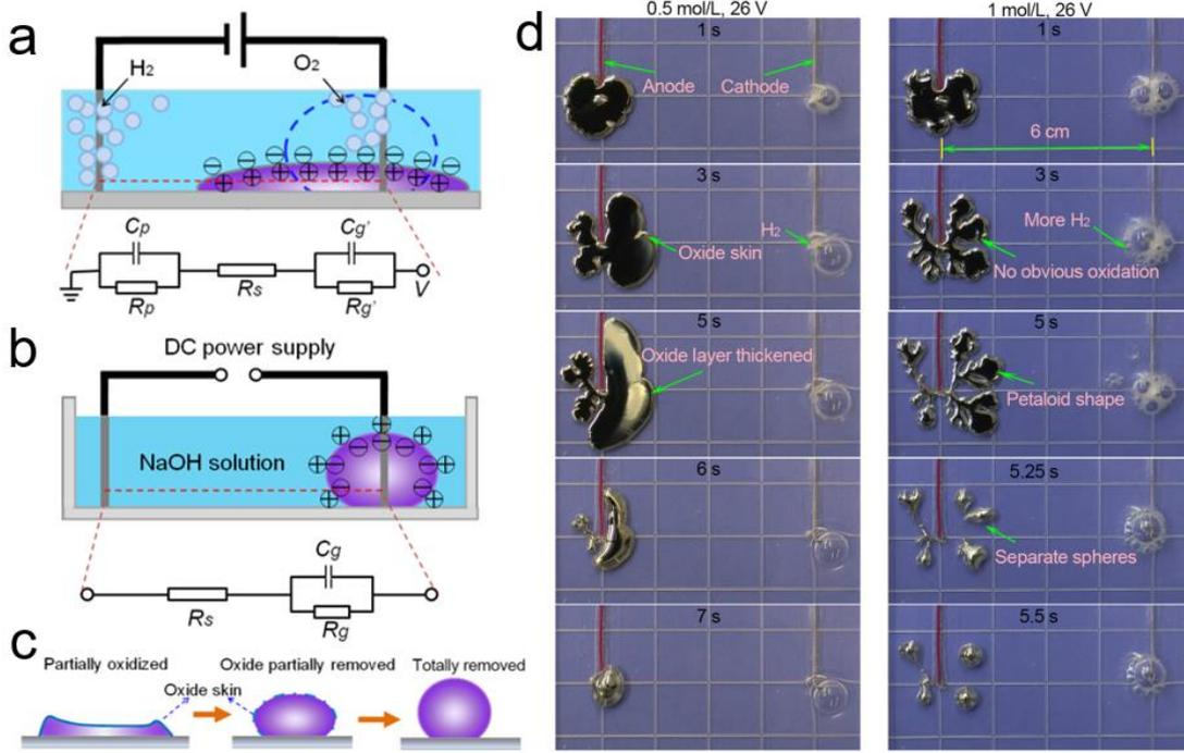
**Figure 10.** Reversible shape and charge redistribution mechanism of liquid metal [35]: (a) Experimental schematic diagram and equivalent circuit after applying DC power; (b) Experimental schematic diagram and equivalent circuit without external power supply; (c) The effect of surface oxide layer on droplet morphology; (d) The change process of the droplet shape when the external power supply was removed after 5s.
