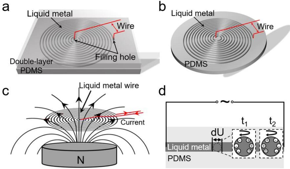
**Figure 3.** Schematic diagrams of liquid metal coil: (a) Method of injection; (b) Method of printing; (c) Magnetic field around the coil; (d) Partial enlarged view of the charge movement and rotation of the liquid metal in the coil.
