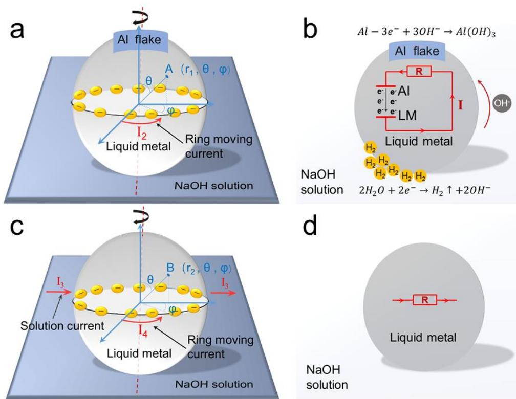
**Figure 11.** Schematic diagram of the movement mechanism and equivalent circuit of surface current in NaOH solution: (a) and (b) liquid metal sphere swallowing aluminum; (c) and (d) Under external electric field.
