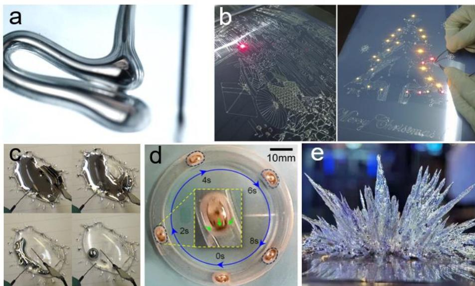
**Figure 2.** Typical material features of liquid metal which may serve to make endogenous magnetic fields: (a) Fluidic behavior; (b) Conductive electronic ink<sup>[21]</sup>; (c) Morphologically transformable machine<sup>[22]</sup>; (d) Self-fueled motor<sup>[23]</sup>; (e) Loadable by magnetic particles<sup>[24]</sup>.
