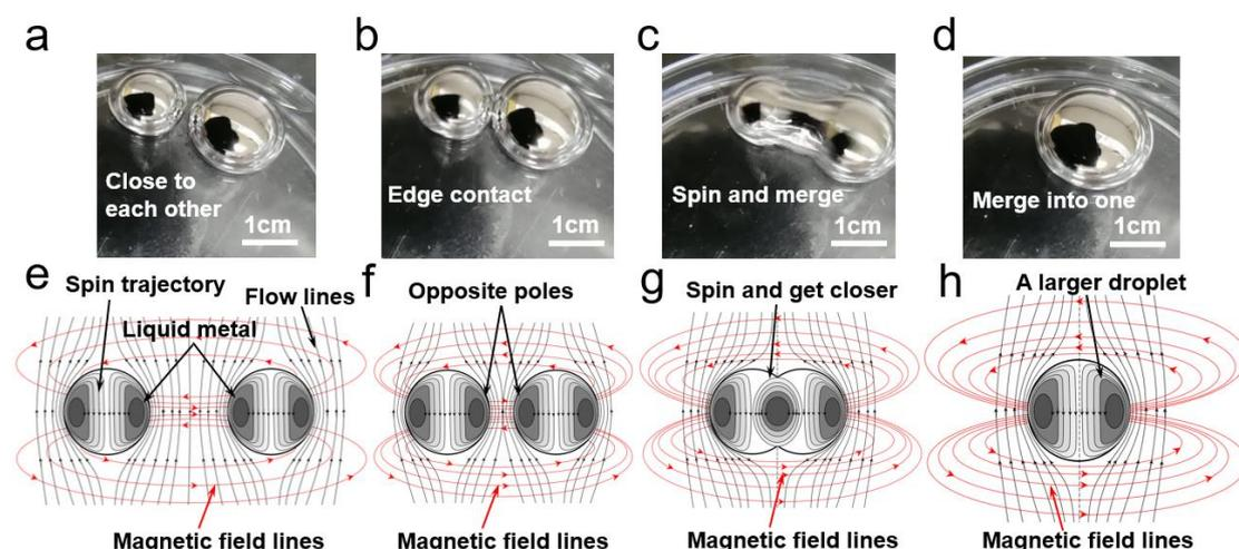
**Figure 7.** Droplets mergence and induced flow and magnetic field: (a-d) Experimental picture of the mergence process of two droplets; (e-h) Spin trajectory of the liquid metal droplets and the surrounding flow lines.
