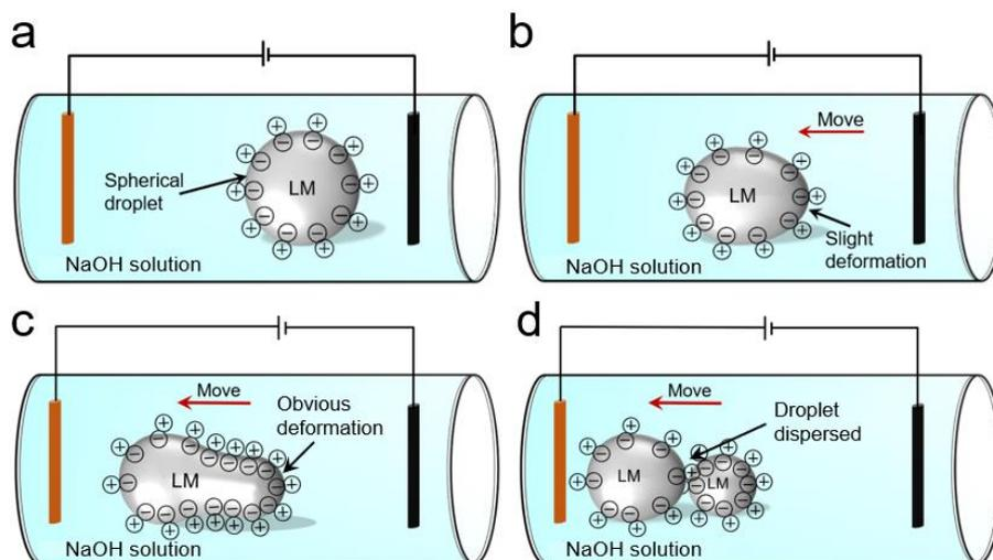
**Figure 4.** The liquid metal droplet continues to move to the electrode under the electric field: (a) The droplet was a regular spherical shape; (b) The droplet moved to the positive electrode with slight deformation; (c) The droplet had obvious head and tail; (d) Droplet dispersed.
