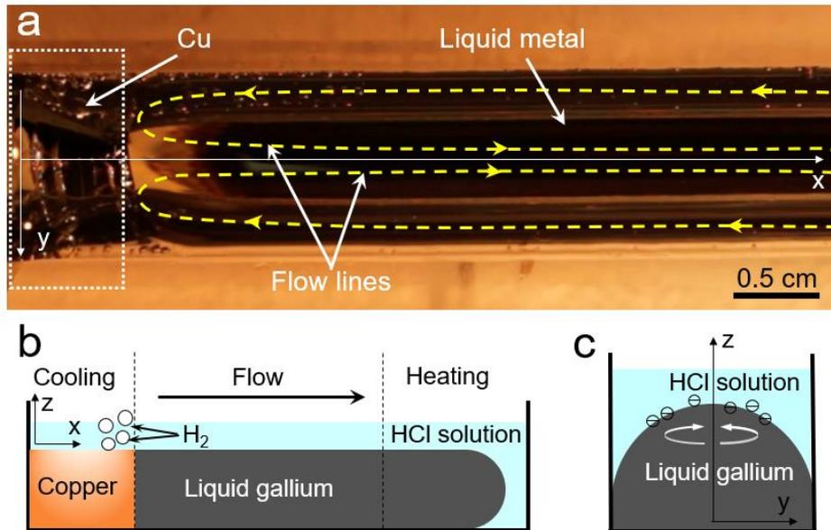
**Figure 9.** Gallium-copper galvanic corrosion: (a) Superficial solution streamline <sup>[34]</sup>; (b) The x-z plan view of galvanic corrosion system in the channel; (c) The y-z plan view of the liquid gallium and HCl solution in the channel.
