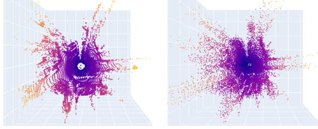
Figure 6: VAE point cloud reconstruction. Left: Original, transformed point cloud. Right: Reconstruction with a bit-rate of 1.83 bpp. The scenery is viewed from above.
