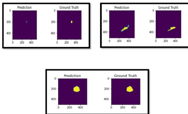
Fig. 5: U-Net: prediction vs ground truth for unseen data
