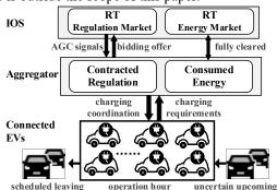
Figure 1. Illustrative schematic of EVA coordination between two sides.
