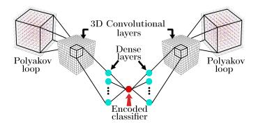
**Figure 1:** Scheme of the autoencoder used in this study. In the encoder, the Polyakov loop configuration is fed into 3D convolutional and then to dense layers; thereby the encoded classifier is obtained. A similar architecture is used for the decoder, which starting from the encoded classifier reconstructs the input configuration.
