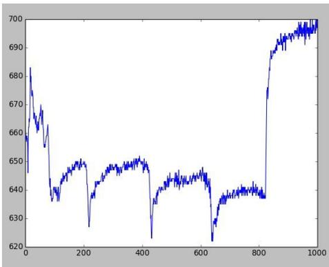
Figure 7. Force sensor values for plastic box 1360 gr.
