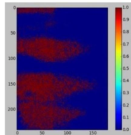
Figure 3. Contact area with noise-filtering.
