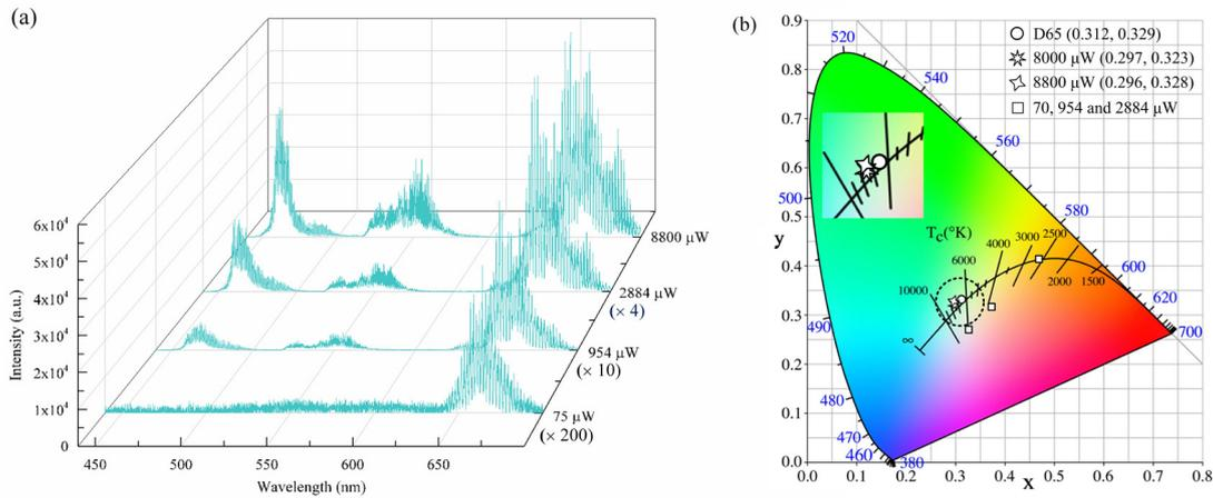
**Figure 3.** a) Lasing spectrum evolution with the increased pump power. b) Plot of the CIE coordinates of standard white illuminant D65 (0.312, 0.329) and lasing spectra under 8000- $\mu\text{W}$  (0.312, 0.329) and 8800- $\mu\text{W}$  (0.296, 0.328) pump powers.
