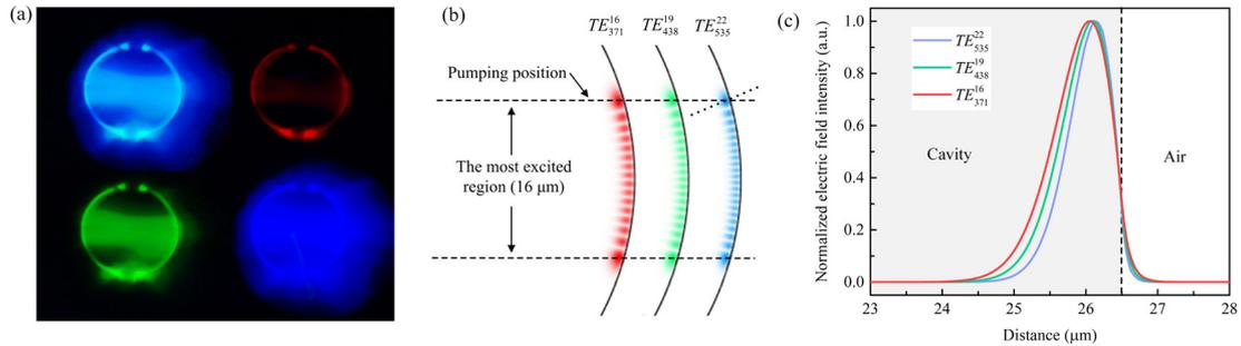
**Figure 4.** a) Optical microscope images of white-like lasing and its component RGB lasing. b) Electric field intensity distributions of  $TE_{371}^{16}$ ,  $TE_{439}^{19}$  and  $TE_{535}^{22}$  modes on the cross-plane of the microsphere along the axis direction, which are calculated by the wavelengths of 460, 560 and 660 nm, respectively.
