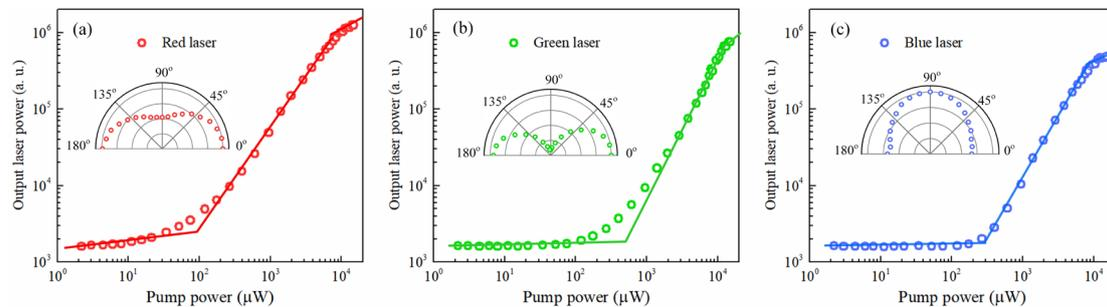
**Figure 2.** a, b, c) Emission intensities of red (a), green (b) and blue (c) lasers versus the pump power in log-log scale, respectively. Their emission intensities are integrated from 619 to 700 nm, 514 to 577 nm, and 446 to 495 nm, respectively. Inset: the emission intensity as a function of the polarization angel.
