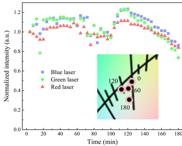
**Figure 5.** a) Lasing intensity evolutions of RGB over the duration of 180 minutes. The inset is the chromaticity of the laser at 0, 60, 120 and 180 minutes.
