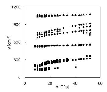
Figure 1. Pressure dependence of bands identified as originating from solid molecular chlorine, taken from one of the experimental runs. Based on ref. [30], we assign these bands as: squares – lattice phonons, circles – intramolecular Cl-Cl vibrations, diamonds – combination modes (Cl-Cl vibration + a lattice phonon), triangles – Cl-Cl vibration overtone. (More detailed information on the assignment can be found in SM.)
