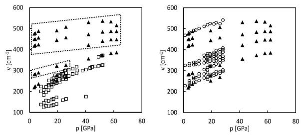
Figure 4. Comparison of new bands appearing in spectra from experiments A and B (solid triangles) with: left panel – known bands from solid chlorine (this work, hollow squares), right panel – known bands from solid CCl<sub>4</sub> (ref. [37], hollow circles). Cl-Cl intramolecular vibron band appearing at 550-600 cm<sup>-1</sup> is omitted for clarity. Dashed parallelograms indicate bands unaccounted for by Cl<sub>2</sub> or CCl<sub>4</sub>.
