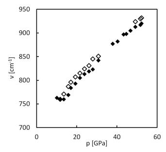
Figure S4. Pressure dependence of one of the combination modes (B<sub>3g</sub> x A<sub>g</sub> = B<sub>3g</sub>) observed in the spectrum of Cl<sub>2</sub>. Filled diamonds – observed frequencies, hollow diamonds – pressure dependence of the sum of frequencies of B<sub>3g</sub> lattice phonon and A<sub>g</sub> Cl<sub>2</sub> vibron. Note the anharmonicity of the observed combination mode, i.e. a lower observed frequency compared to the simple sum.
