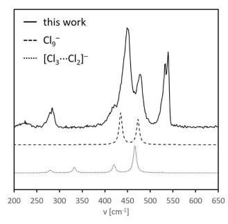
Figure 6. Comparison of the 200-600 cm<sup>-1</sup> region of sample B spectra at 3.9 GPa with Raman bands of polychloride anions derived from ref. [38] for Cl<sub>9</sub><sup>-</sup> anion and from ref. [39] for 2D polychloride network. Relative intensities are also adapted from cited works.
