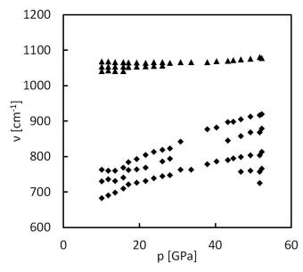
Figure S3. Pressure dependence of bands designated as originating from  $Cl_2$  in the 600-1200 cm<sup>-1</sup> range – this work.
