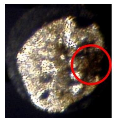
Figure S6. Picture of sample from experiment A after initial compression and laser heating. Note the brown color of the irradiated spot.
