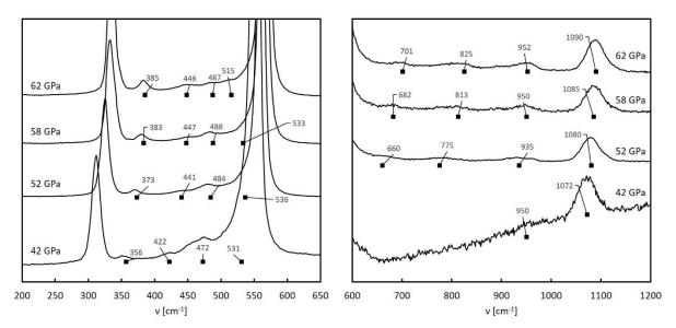
Figure 2. Comparison of spectra obtained in experiment A: AgCl + Cl<sub>2</sub> mixture compressed initially to ca. 40 GPa. See text for further details.
