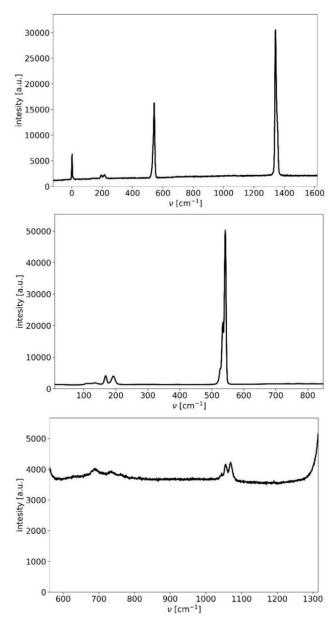
Fig. S1. Spectra of solid chlorine obtained at 8 GPa. The high-intensity band at ca. 1350 cm<sup>-1</sup> originated from diamond anvil.
