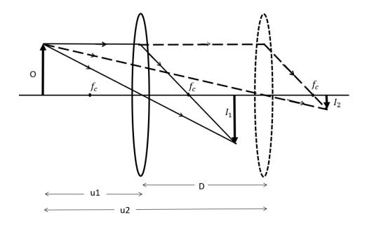
Fig.1 Image formation at the two positions of the lens  $\,$
