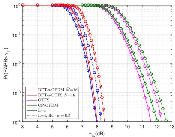
(d) PAPR for discrete and continuous time of DFT-s-OFDM, DFT-s-OTFS, OTFS, and CP-OFDM ( $M=64$  and  $N=32$ ).
