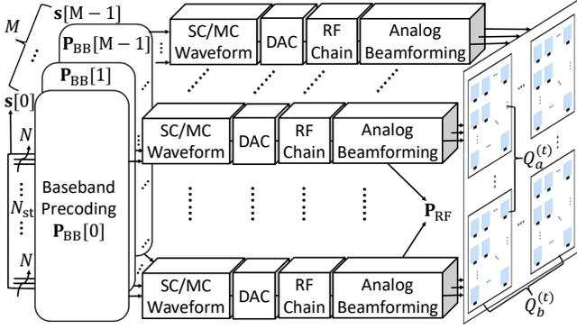
Fig. 1: Block diagram of a THz-band UM-MIMO transmitter.
