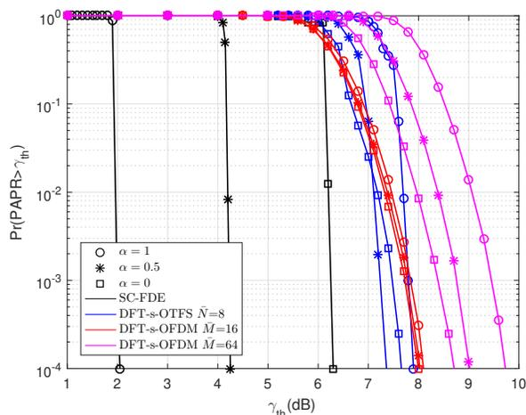
(c) Effect of pulse-shaping for SC waveforms ( $M=128$  and  $N=16$ ).
