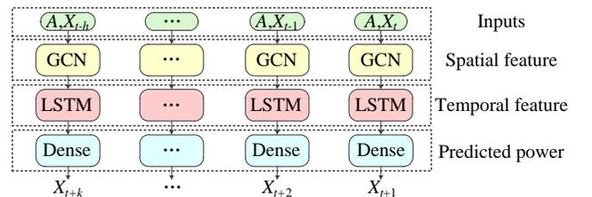
Figure 1. The framework of the proposed method.
