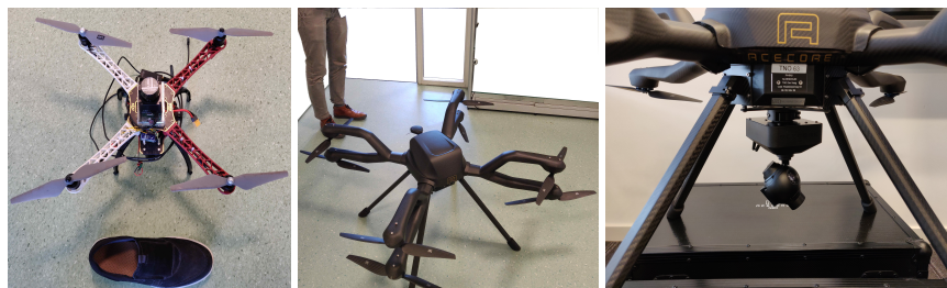
Fig. 1 Examples of the drones available at the Intelligent Autonomous Systems group at TNO: (left) a small device for proof of concept testing, shoe for scale. (center) a heavy-duty AceCore NEO drone. (right) a bottom mounted gimbal for visual data collection, possibly to be analyzed onboard for fast victim recognition.
