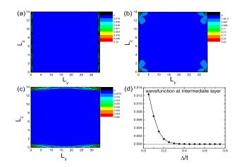
FIG. 4. The evolutions of wavefunctions for the chiral Majorana edge modes as the superconducting gap  $\Delta$  is adjusted. The parameters are  $\Gamma/t = 1.0$  and  $\Delta/t = 0.02$ , 0.65, 0.80 in (a)-(c).
