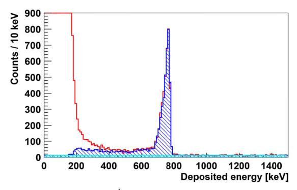
**Figure 3**. Spectrum measured in the <sup>3</sup>He thermal detector (red line). The peak at low energy is due to electronic noise and  $\gamma$ -ray background, while the neutron-detection peak is visible at 764 keV. The blue dash-filled line is the *pure* neutron response from a measurement with <sup>252</sup>Cf. The cyan dot-filled line is the linear background from the intrinsic  $\alpha$ -radioactivity of the counter.
