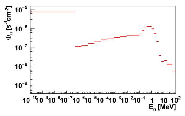
**Figure 4**. Energy distribution of the neutron flux obtained with the EM method, the response of figure 2 rebinned in 24 bins as in [7] and a *prior* distribution defined using functions from [11].
