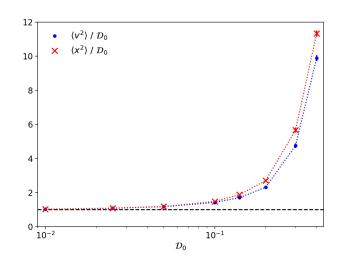
Figure 2. For a harmonic potential with  $\Omega = 0.1$ ,  $\langle v^2 \rangle / \mathcal{D}_0$  and  $\langle x^2 \rangle / \mathcal{D}_0$  as a function of  $\mathcal{D}_0$  ( $\mathcal{D}_1 = 0$ ). For  $\mathcal{D}_0 \to 0$  equipartition is approximately valid while it is violated for  $0.1 \leq \mathcal{D}_0$ . Dotted lines are guides to the eye.
