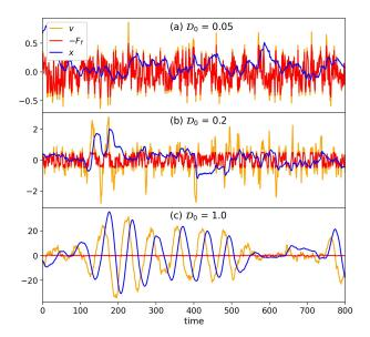
Figure 1. Example of time series of velocity, minus friction force, and position, for a harmonic potential with  $\Omega = 0.1$ ,  $D_1 = 0$  and (a)  $D_0 = 0.05$ , (b)  $D_0 = 0.2$ , (c)  $D_0 = 1$ . Numerical integrations of (16) follow the scheme (30) with  $dt \leq 10^{-4}$ .
