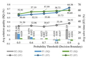
Fig. 3. B1-Normalized solution quality (SQ) and solve time (ST) averaged over test samples in percent for IEEE 24-Bus system with respect to decision boundary.
