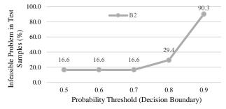
Fig. 2. Test sample infeasibility in IEEE 24-Bus system for B2.
