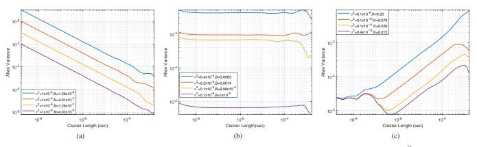
Figure 3: (a) Synthesized white noise (b) flicker noise and (c) random walk noise with different  $\sigma^2$  values
