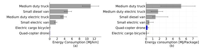
Figure 2: Energy Consumption for different transportation modes. Error bars represent variations in (a) driving styles and vehicle characteristics, and (b) number of packages delivered per distance.
