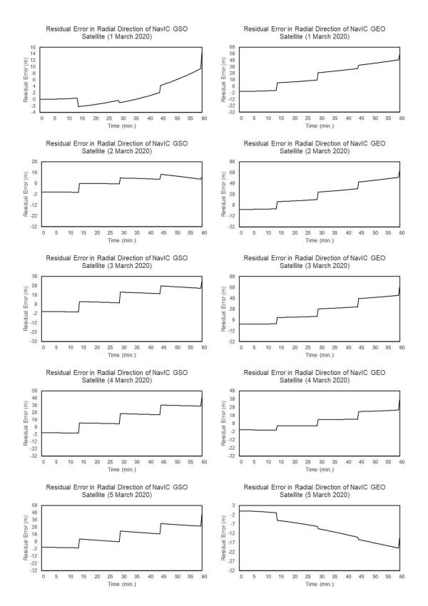
Figure 1: Residual Error in Radial Direction of NavIC satellites predicted using UKF
