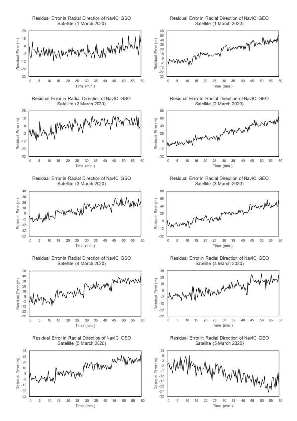
Figure 2: Residual Error in Radial Direction of NavIC satellites predicted using BPF
