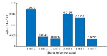
Fig. 3. Asymptotic KL rate metric between the original model cM0 and all  $\mathcal{M}_i$ . Each  $\mathcal{M}_i$  corresponds to truncation of two states from set S. Higher values of KL rate metric indicate larger difference between the models.
