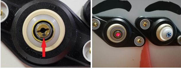
FIG. 2. Two simultaneously actuated spherical bearings (25 mm in diam) host a laser pointer and a microcamera, respectively. A magnet (red arrow in the close-up image at left) is applied in the proximity of the laser output window and is localized by the tracking system. The bearings reproduce motion of the eyes and are mounted on a movable frame that represents the head. *link VIDEO1* (Multimedia view)
