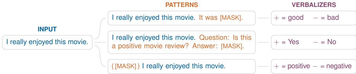
Figure 2: Different choices of patterns and corresponding verbalizers for classifying movie reviews as positive (+) or negative (-). The input is first converted into a cloze question using the pattern; classification is done by computing the output whose verbalization is the most likely substitute for the mask according to the MLM.
