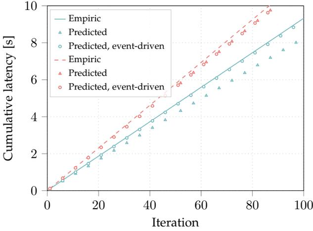
Fig. 6: Cumulative latency over 100 iterations. Blue curves correspond to  $w = 9$  and red curves to  $w = 72$ . Each iteration ends once  $w$  workers have completed their task. For  $w < N$ , we need to account for the case where workers remain unavailable over several iterations, which we do using the model based on event-driven simulations.
