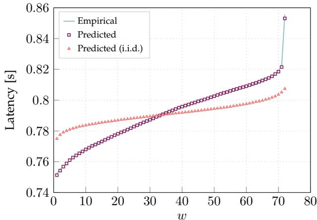
Fig. 5: Average latency of the  $w$ -th fastest worker out of  $N = 72$  workers for a computation on Azure, and predicted latency, where the per-worker latency is modeled as either independent, but not necessarily identically distributed, or i.i.d., between workers. The i.i.d. assumption can significantly reduce accuracy.
