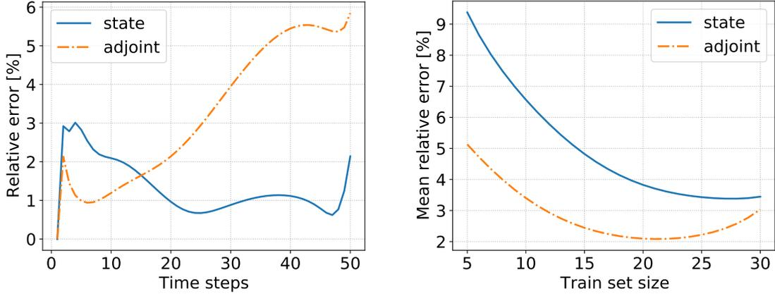
Figure 2: On the left the  $L^2$  relative reconstruction error for the Graetz case for state and adjoint variables. On the right the  $L^2$  mean relative prediction error. The average is done over 20 snapshots in the future.
