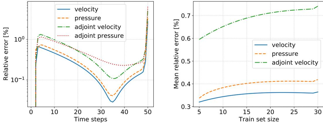
Figure 3: On the left the  $L^2$  relative reconstruction error for the Stokes case for velocity, pressure, and the adjoint variables. On the right the  $L^2$  mean relative prediction error. The average is done over 20 snapshots in the future.
