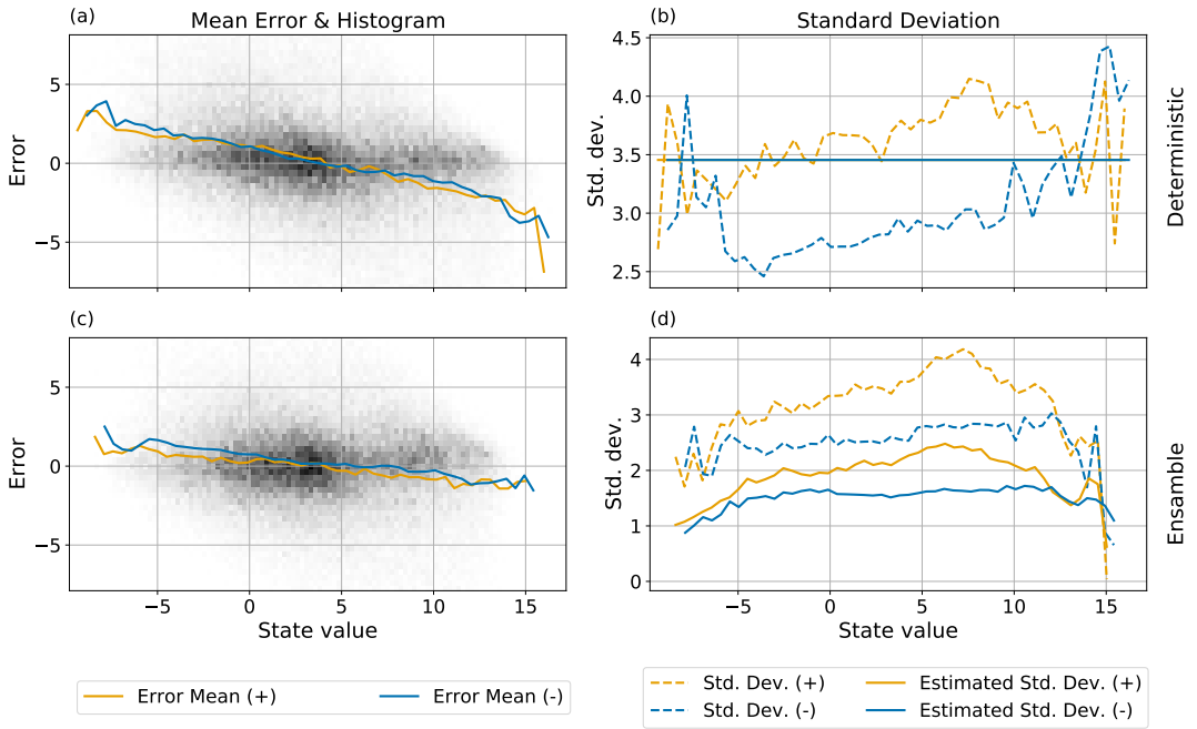
FIGURE 10 Panels (a) and (c) show the 2D density of the forecast error and forecasted state values (grey shades). The yellow and blue solid lines indicates the mean forecast error as a function of the forecasted state value for the positive trend and negative trend sub-samples respectively (see the text for details). Panels (b) and (d) show the standard deviation of the error as function of the forecasted state variable for the positive trend and negative trend sub-samples (dashed yellow line and dashed blue line respectively). The solid yellow and blue lines represents the estimated standard deviation for the positive trend and negative trends sub-samples respectively. Panels (a) and (b) corresponds to the deterministic forecast and (c) and (d) to the ensemble forecast. All panels corresponds to the imperfect model scenario.
