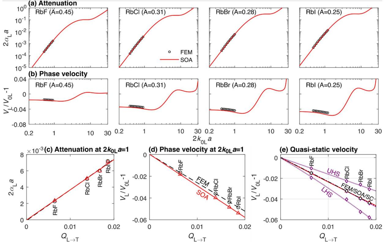
Figure 7. (a) Normalised attenuation and (b) phase velocity variation versus normalised frequency for plane longitudinal waves in four cubic polycrystals with the PVT microstructure and  $A < 1$ , comparing the SOA and FEM results. (c) and (d) show the normalised attenuation and velocity variation at  $2k_{0L} a = 1$  against the elastic scattering factor  $Q_{L \rightarrow T}$ . (e) displays the velocity variation at the quasi-static limit.
