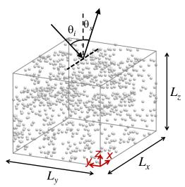
Fig. 1. Simulation setup composed of  $N_p$  particles randomly arranged inside a rectangular region with dimensions  $L_x$ ,  $L_y$ , and  $L_z$ . The structure is illuminated by a plane wave propagating in the xz-plane with the incident angle of  $\theta_i$ . The area between the dielectric particles is filled with air and the scattering is calculated in the upper half plane for  $-\pi/2 \le \theta_s \le \pi/2$ .
