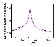
Fig. 5. Numerically calculated normalized ensemble-averaged scattering intensity for  $N_p = 10000$ ,  $L = 20\lambda_0$ , and  $\rho = 0.021$  for  $N_r = 10000$  (dark curve) and theoretical fit (Eq. (3)) with  $l_e$  used as fitting parameter (light color). Note that  $l_e$  value is normalized to the free-space wavelength.
