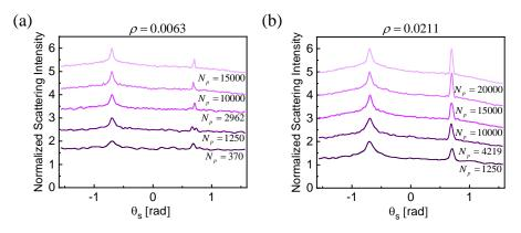
Fig. 7. Normalized ensemble-averaged scattering intensity for two different density factors  $\rho$  while the number of particles and the size of the enclosing box are changed. Curves correspond
