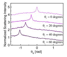
Fig. 4. Elimination of specular reflection from ensemble-averaged scattered intensity. Random samples are similar with those used in Fig. 3, where an artificial random surface is added on top of the medium shown in Fig. 1. The angle of incidence is set at  $\theta_i = (60, 40, 20, 0)$  [deg]
