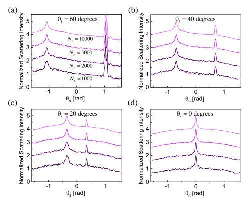
Fig. 3. Normalized ensemble-averaged scattering intensity for random samples with  $N_p = 10000$ ,  $L = 20\lambda_p$ , and  $\rho = 0.021$ . Results are averaged over
