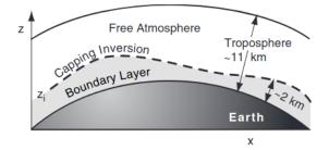
Figure 1: A schematic diagram of the PBL shown as a vertical cross section of the Earth and troposphere, where the PBL occupies the lowest portion of the latter (Stull, 2017).
