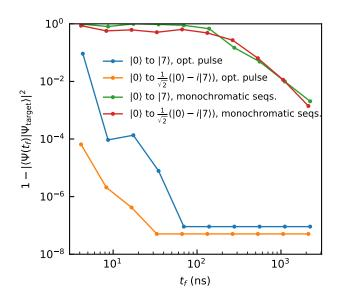
FIG. 3. Infidelities for the  $|0\rangle \rightarrow |7\rangle$  and  $|0\rangle \rightarrow \frac{1}{\sqrt{2}}(|0\rangle - i|7\rangle)$  transitions, as a function of operation time, for the pulses obtained as a sequence of monochromatic resonant pulses ( $\pi$  or  $\pi/2$ ), and for the optimal pulses obtained with QOCT.
