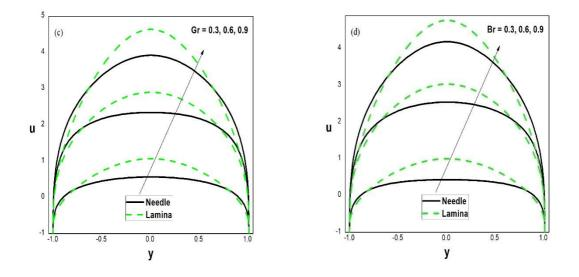
Figures2(c)-(d): variation of velocity profile versus y.when b = 0.5, t = 0.2, x = 0.2, a = 0.5, d = 1.5, Sr = 0.8, Nt = 0.6,  $Q_1 = 1.5$ , Nb = 0.6,  $\beta_2 = 1.2$ ,  $\beta_3 = 1.2$  and  $\omega = 0.7$ . (c) Br = 0.8,  $\beta = 0.7$  and  $\beta_1 = 1.2$ . (d) Gr = 0.8,  $\beta = 0.7$ ,  $\beta_1 = 1.2$ .
