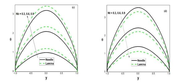
Figures3(c)-(d): variation of temperature profile versus y.when b = 0.5, t = 0.2, x = 0.2, a = 0.5,  $\beta_3 = 1.2$ , d = 1.5 and  $\omega = 0.7$ . (c) Nt = 0.6,  $Q_1 = 1.5$ ,  $\beta_2 = 1.2$  and Sr = 0.8. (d)  $\beta_2 = 1.2$ ,  $Q_1 = 1.5$ , Nb = 0.6 and Sr = 0.8.
