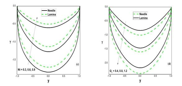
Figures4(c)-(d): variation of nanoparticle concentration versus y.when b = 0.5, t = 0.2, x = 0.2, Sr = 0.8, a = 0.5,  $\beta_2 = 1.2$ , d = 1.5 and  $\omega = 0.7$ . (c)  $\beta_3 = 1.2$ , Nb = 0.6 and  $Q_1 = 1.5$ . (d) Nt = 0.6, Nb = 0.6 and  $\beta_3 = 1.2$ .
