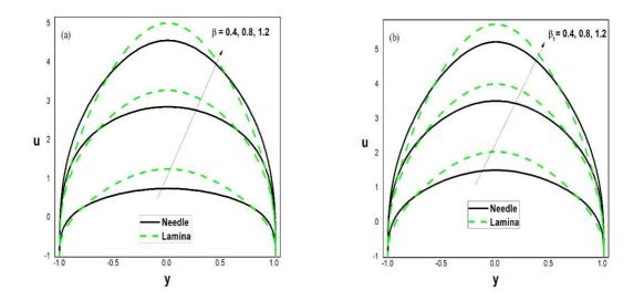
Figures2(a)-(b): variation of velocity profile versus y.when b = 0.5, t = 0.2, x = 0.2, a = 0.5, d = 1.5, Sr = 0.8, Nt = 0.6,  $Q_1 = 1.5$ , Nb = 0.6,  $\beta_2 = 1.2$ ,  $\beta_3 = 1.2$  and  $\omega = 0.7$ . (a) Br = 0.8, Gr = 0.8 and  $\beta_1 = 1.2$ . (b) Br = 0.8, Gr = 0.8 and  $\beta = 0.7$ .
