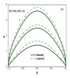
Figure 3(e): variation of temperature profile versus y.when b = 0.5, t = 0.2, x = 0.2, a = 0.5,  $\beta_3 = 1.2$ , d = 1.5and  $\omega = 0.7$ . (e) Nt = 0.6,  $\beta_2 = 1.2$ , Nb = 0.6 and Sr = 0.8.
