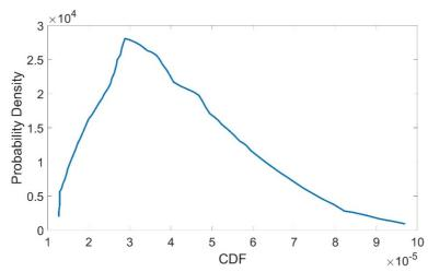
Fig. 4. Calculated CDF distribution of a generic PWR (W) with the following uncertainty statistics: mean 3.9 10<sup>-5</sup>, standard deviation 1.6 10<sup>-5</sup>, and 5<sup>th</sup> and 95<sup>th</sup> percentiles 1.7 10<sup>-5</sup> and 7 10<sup>-5</sup> respectively.
