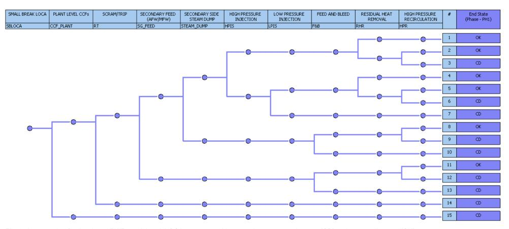
Fig. 1. An example of a developed PWR small-break LOCA event tree with two end-states: core damage (CD) and no core damage (OK)
