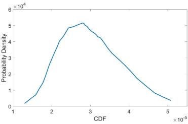
Fig. 5. Calculated CDF distribution of a typical GE BWR-4 design with the following uncertainty statistics: mean  $2.9\ 10^{-5}$ , standard deviation  $7.8\ 10^{-6}$ , and  $5^{th}$  and  $95^{th}$  percentiles  $1.8\ 10^{-5}$  and  $4.3\ 10^{-5}$  respectively.
