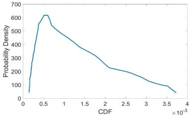
Fig. 7. CCDP distribution of a GE BWR LOOP event concurrent with an EDG unavailability
