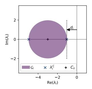
FIG. 1. Negative margins  $d_i$  ensure linear stability of the voltage subsystem: The voltage subsystem of N =2 coupled third-order synchronous machines is evaluated in terms of the margin  $d_i$ . The two Gershgorin disks coincide, and the true positions of the eigenvalues are precisely on the borders of the disks. The parameters are  $P_1 = -P_2 = 1.5$ ,  $B_{12} = B_{21} = 2$ ,  $E^f = 2$ , 1.0 and  $\Gamma_1 = \Gamma_2 = 0$ .
