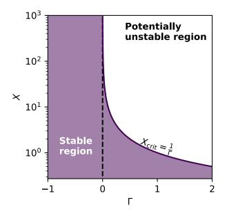
FIG. 2. The minimal stable region of the voltage subsystem depends on the parameter  $\Gamma$ : The matrix of the voltage subsystem is negative definite in the purple region, such that no pure voltage instability occurs here. In particular, for  $\Gamma \leq 0$  the voltage subsystem alone is linearly stable for all  $X \in \mathbb{R}^+$ . This analysis holds for arbitrary system sizes N, parameter settings and thus network topologies.
