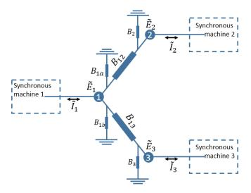
FIG. 3. Sample grid to explain the properties of the nodal susceptance matrix B: The sample grid consists of three interconnected machines. The variables  $\tilde{E}_i$  stand for the voltage at the respective node. The variables  $\tilde{I}_i$  represent the current that flows from each node to the attached dashed box.
