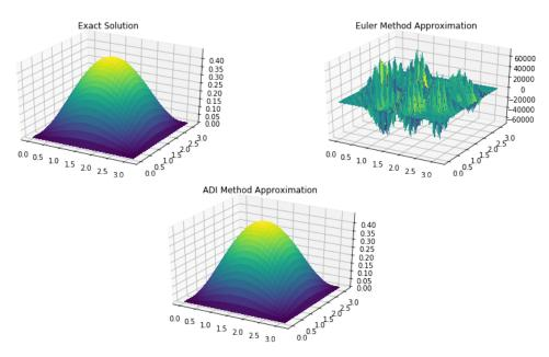
Figure 2.7. Euler vs ADI approximation with  $L = \pi, dt = 0.02, dx = dy = 0.1, T = 0.2$
