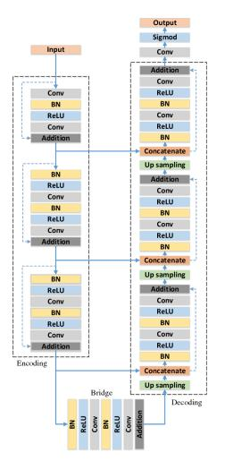
Figure 2.3. The architecture of the proposed deep ResUnet. [9]
