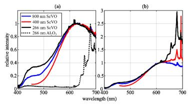
Fig. 4. Normalized emission spectra (0.3 nm resolution) of (a) ScVO<sub>4</sub>:Bi<sup>3+</sup> (under the MPE and SPE schemes) and alumina, (b) ScVO<sub>4</sub>:Bi<sup>3+</sup> coated on an alumina substrate.
