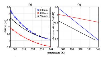
Fig. 5. (a) ScVO<sub>4</sub>:Bi<sup>3+</sup> lifetime vs. temperature. Solid lines represent a data fit. (b) Relative temperature sensitivity vs. evaluation from the respective fit.
