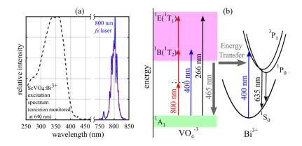
Fig. 2. (a) Excitation spectrum of ScVO<sub>4</sub>:Bi<sup>3+</sup> (data plotted with permission of Phosphor Technology, UK) and spectrum for the fs 800 nm laser light (red-dash line is a fit), (b) Schematic configuration coordinate diagram for ScVO<sub>4</sub>:Bi<sup>3+</sup>.
