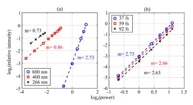
Fig. 3. Natural log-log plots of phosphorescence intensity versus excitation average power, (a) for each scheme, (b) for different pulse durations (FWHM) with 800 nm excitation.
